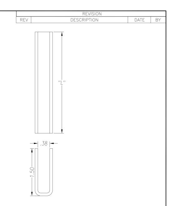
FOR LENGTH DIMENSION ("L"), SEE PURCHASE ORDER. LENGTH TOLERANCE:LESS THAN 60":  $\pm 1/16$ " LESS THAN 120":  $\pm 1/8$ ", 120" OR GREATER:  $\pm 1/4$ " MAXIMUM BURR NOT TO EXCEED 10% OF MAT'L THICKNESS WITH THE EXCEPTION OF CUT ENDS, WHICH MAY HAVE BURR EXCEEDING THIS AMOUNT. FINISHED PART MAY EXHIBIT TYPICAL ROLL FORMED END FLARE UP TO THREE INCHES FROM ENDS. PROFILE DIMENSIONS TO BE MEASURED 3" OR GREATER FROM CUT ENDS.
