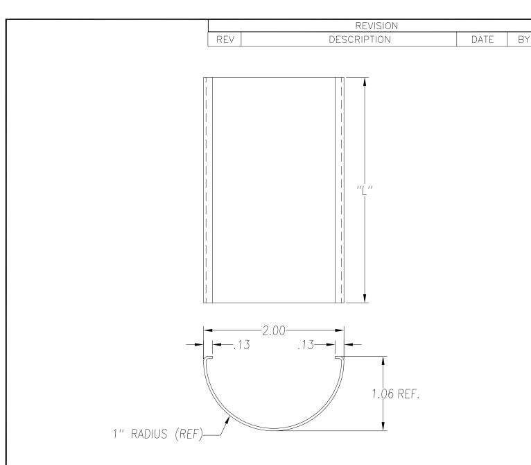
FOR LENGTH DIMENSION ("L"), SEE PURCHASE ORDER. LENGTH TOLERANCE:LESS THAN 60":  $\pm 1/16$ " LESS THAN 120":  $\pm 1/8$ ", 120" OR GREATER:  $\pm 1/4$ " MAXIMUM BURR NOT TO EXCEED 10% OF MAT'L THICKNESS WITH THE EXCEPTION OF CUT ENDS, WHICH MAY HAVE BURR EXCEEDING THIS AMOUNT. FINISHED PART MAY EXHIBIT TYPICAL ROLL FORMED END FLARE UP TO THREE INCHES FROM ENDS. PROFILE DIMENSIONS TO BE MEASURED 3" OR GREATER FROM CUT ENDS.
