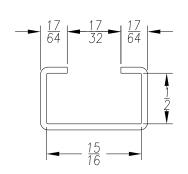
FOR LENGTH DIMENSION ("L"), SEE PURCHASE ORDER. LENGTH TOLERANCE:LESS THAN 60":  $\pm 1/16$ " LESS THAN 120":  $\pm 1/8$ ", 120" OR GREATER:  $\pm 1/4$ " MAXIMUM BURR NOT TO EXCEED 10% OF MAT'L THICKNESS WITH THE EXCEPTION OF CUT ENDS, WHICH MAY HAVE BURR EXCEEDING THIS AMOUNT. FINISHED PART MAY EXHIBIT TYPICAL ROLL FORMED END FLARE UP TO THREE INCHES FROM ENDS. PROFILE DIMENSIONS TO BE MEASURED 3" OR GREATER FROM CUT ENDS.
