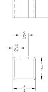
FOR LENGTH DIMENSION ("L"), SEE PURCHASE ORDER. LENGTH TOLERANCE:LESS THAN 60":  $\pm 1/16$ " LESS THAN 120":  $\pm 1/8$ ", 120" OR GREATER:  $\pm 1/4$ " MAXIMUM BURR NOT TO EXCEED 10% OF MAT'L THICKNESS WITH THE EXCEPTION OF CUT ENDS, WHICH MAY HAVE BURR EXCEEDING THIS AMOUNT. FINISHED PART MAY EXHIBIT TYPICAL ROLL FORMED END FLARE UP TO THREE INCHES FROM ENDS. PROFILE DIMENSIONS TO BE MEASURED 3" OR GREATER FROM CUT ENDS.
