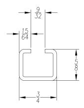
FOR LENGTH DIMENSION ("L"), SEE PURCHASE ORDER. LENGTH TOLERANCE:LESS THAN 60":  $\pm 1/16$ " LESS THAN 120":  $\pm 1/8$ ", 120" OR GREATER:  $\pm 1/4$ " MAXIMUM BURR NOT TO EXCEED 10% OF MAT'L THICKNESS WITH THE EXCEPTION OF CUT ENDS, WHICH MAY HAVE BURR EXCEEDING THIS AMOUNT. FINISHED PART MAY EXHIBIT TYPICAL ROLL FORMED END FLARE UP TO THREE INCHES FROM ENDS. PROFILE DIMENSIONS TO BE MEASURED 3" OR GREATER FROM CUT ENDS.
