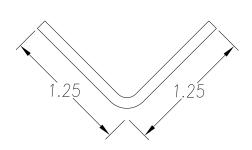
FOR LENGTH DIMENSION ("L"), SEE PURCHASE ORDER. LENGTH TOLERANCE:LESS THAN 60":  $\pm 1/16$ " LESS THAN 120":  $\pm 1/8$ ", 120" OR GREATER:  $\pm 1/4$ " MAXIMUM BURR NOT TO EXCEED 10% OF MAT'L THICKNESS WITH THE EXCEPTION OF CUT ENDS, WHICH MAY HAVE BURR EXCEEDING THIS AMOUNT. FINISHED PART MAY EXHIBIT TYPICAL ROLL FORMED END FLARE UP TO THREE INCHES FROM ENDS. PROFILE DIMENSIONS TO BE MEASURED 3" OR GREATER FROM CUT ENDS.
