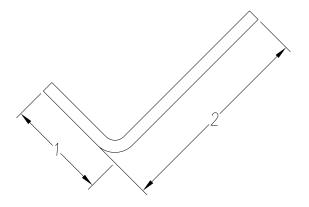
SEE PO FOR MATERIAL TYPE AND FINISH FOR LENGTH DIMENSION ("L"), SEE PURCHASE ORDER. LENGTH TOLERANCE:LESS THAN 60":  $\pm 1/16$ " LESS THAN 120":  $\pm 1/8$ ", 120" OR GREATER:  $\pm 1/4$ " MAXIMUM BURR NOT TO EXCEED 10% OF MAT'L THICKNESS WITH THE EXCEPTION OF CUT ENDS, WHICH MAY HAVE BURR EXCEEDING THIS AMOUNT. FINISHED PART MAY EXHIBIT TYPICAL ROLL FORMED END FLARE UP TO THREE INCHES FROM ENDS. PROFILE DIMENSIONS TO BE MEASURED 3" OR GREATER FROM CUT ENDS.
