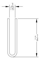
SEE PO FOR MATERIAL TYPE AND FINISH FOR LENGTH DIMENSION ("L"), SEE PURCHASE ORDER. LENGTH TOLERANCE:LESS THAN 60":  $\pm 1/16$ " LESS THAN 120":  $\pm 1/8$ ", 120" OR GREATER:  $\pm 1/4$ " MAXIMUM BURR NOT TO EXCEED 10% OF MAT'L THICKNESS WITH THE EXCEPTION OF CUT ENDS, WHICH MAY HAVE BURR EXCEEDING THIS AMOUNT. FINISHED PART MAY EXHIBIT TYPICAL ROLL FORMED END FLARE UP TO THREE INCHES FROM ENDS. PROFILE DIMENSIONS TO BE MEASURED 3" OR GREATER FROM CUT ENDS.
