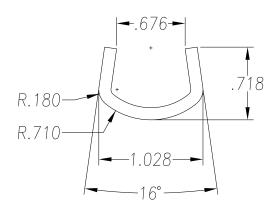
SEE PO FOR MATERIAL TYPE AND FINISH FOR LENGTH DIMENSION ("L"), SEE PURCHASE ORDER. LENGTH TOLERANCE:LESS THAN 60": ±1/16" LESS THAN 120": ±1/8", 120" OR GREATER: ± 1/4" MAXIMUM BURR NOT TO EXCEED 10% OF MAT'L THICKNESS WITH THE EXCEPTION OF CUT ENDS, WHICH MAY HAVE BURR EXCEEDING THIS AMOUNT. FINISHED PART MAY EXHIBIT TYPICAL ROLL FORMED END FLARE UP TO THREE INCHES FROM ENDS. PROFILE DIMENSIONS TO BE MEASURED 3" OR GREATER FROM CUT ENDS.
