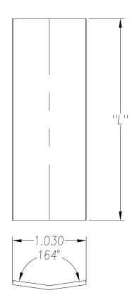
SEE PO FOR MATERIAL TYPE AND FINISH FOR LENGTH DIMENSION ("L"), SEE PURCHASE ORDER. LENGTH TOLERANCE:LESS THAN 60":  $\pm 1/16$ " LESS THAN 120":  $\pm 1/8$ ", 120" OR GREATER:  $\pm 1/4$ " MAXIMUM BURR NOT TO EXCEED 10% OF MAT'L THICKNESS WITH THE EXCEPTION OF CUT ENDS, WHICH MAY HAVE BURR EXCEEDING THIS AMOUNT. FINISHED PART MAY EXHIBIT TYPICAL ROLL FORMED END FLARE UP TO THREE INCHES FROM ENDS. PROFILE DIMENSIONS TO BE MEASURED 3" OR GREATER FROM CUT ENDS.
