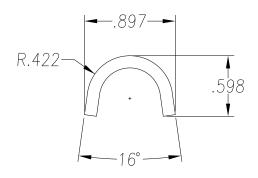
SEE PO FOR MATERIAL TYPE AND FINISH FOR LENGTH DIMENSION ("L"), SEE PURCHASE ORDER. LENGTH TOLERANCE:LESS THAN 60":  $\pm 1/16$ " LESS THAN 120":  $\pm 1/8$ ", 120" OR GREATER:  $\pm 1/4$ " MAXIMUM BURR NOT TO EXCEED 10% OF MAT'L THICKNESS WITH THE EXCEPTION OF CUT ENDS, WHICH MAY HAVE BURR EXCEEDING THIS AMOUNT. FINISHED PART MAY EXHIBIT TYPICAL ROLL FORMED END FLARE UP TO THREE INCHES FROM ENDS. PROFILE DIMENSIONS TO BE MEASURED 3" OR GREATER FROM CUT ENDS.
