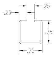
SEE PO FOR MATERIAL TYPE AND FINISH FOR LENGTH DIMENSION ("L"), SEE PURCHASE ORDER. LENGTH TOLERANCE:LESS THAN 60":  $\pm 1/16$ " LESS THAN 120":  $\pm 1/8$ ", 120" OR GREATER:  $\pm 1/4$ " MAXIMUM BURR NOT TO EXCEED 10% OF MAT'L THICKNESS WITH THE EXCEPTION OF CUT ENDS, WHICH MAY HAVE BURR EXCEEDING THIS AMOUNT.
