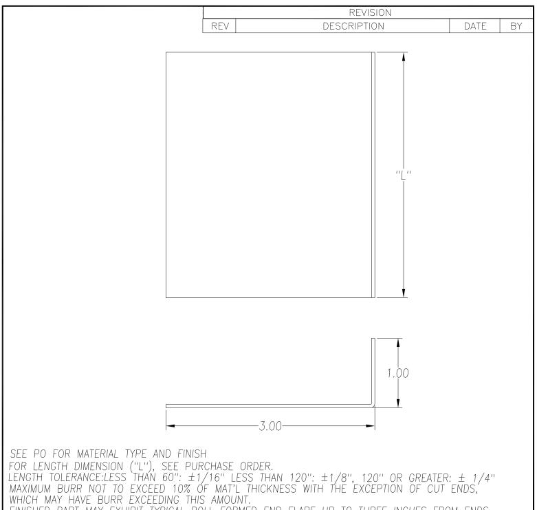
FINISHED PART MAY EXHIBIT TYPICAL ROLL FORMED END FLARE UP TO THREE INCHES FROM ENDS. PROFILE DIMENSIONS TO BE MEASURED 3" OR GREATER FROM CUT ENDS.
