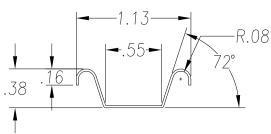
SEE PO FOR MATERIAL TYPE AND FINISH FOR LENGTH DIMENSION ("L"), SEE PURCHASE ORDER. LENGTH TOLERANCE:LESS THAN 60":  $\pm 1/16$ " LESS THAN 120":  $\pm 1/8$ ", 120" OR GREATER:  $\pm 1/4$ " MAXIMUM BURR NOT TO EXCEED 10% OF MAT'L THICKNESS WITH THE EXCEPTION OF CUT ENDS, WHICH MAY HAVE BURR EXCEEDING THIS AMOUNT. FINISHED PART MAY EXHIBIT TYPICAL ROLL FORMED END FLARE UP TO THREE INCHES FROM ENDS. PROFILE DIMENSIONS TO BE MEASURED 3" OR GREATER FROM CUT ENDS.
