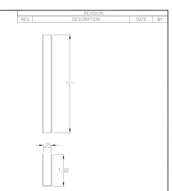
SEE PO FOR MATERIAL TYPE AND FINISH FOR LENGTH DIMENSION ("L"), SEE PURCHASE ORDER. LENGTH TOLERANCE:LESS THAN 60":  $\pm 1/16$ " LESS THAN 120":  $\pm 1/8$ ", 120" OR GREATER:  $\pm 1/4$ " MAXIMUM BURR NOT TO EXCEED 10% OF MAT'L THICKNESS WITH THE EXCEPTION OF CUT ENDS, WHICH MAY HAVE BURR EXCEEDING THIS AMOUNT. FINISHED PART MAY EXHIBIT TYPICAL ROLL FORMED END CUT DISTORTION. PROFILE DIMENSIONS TO BE MEASURED 2" OR GREATER FROM CUT ENDS.
