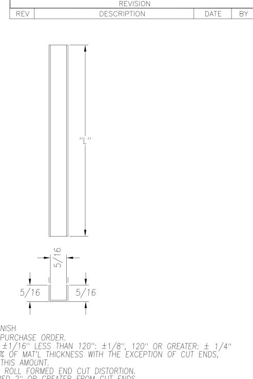
SEE PO FOR MATERIAL TYPE AND FINISH FOR LENGTH DIMENSION ("L"), SEE PURCHASE ORDER. LENGTH TOLERANCE:LESS THAN 60":  $\pm 1/16$ " LESS THAN 120":  $\pm 1/8$ ", 120" OR GREATER:  $\pm 1/4$ " MAXIMUM BURR NOT TO EXCEED 10% OF MAT'L THICKNESS WITH THE EXCEPTION OF CUT ENDS, WHICH MAY HAVE BURR EXCEEDING THIS AMOUNT. FINISHED PART MAY EXHIBIT TYPICAL ROLL FORMED END CUT DISTORTION. PROFILE DIMENSIONS TO BE MEASURED 2" OR GREATER FROM CUT ENDS.
