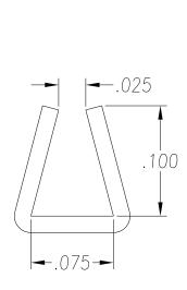
SEE PO FOR MATERIAL TYPE AND FINISH FOR LENGTH DIMENSION ("L"), SEE PURCHASE ORDER. LENGTH TOLERANCE:LESS THAN 60": ±1/16" LESS THAN 120": ±1/8", 120" OR GREATER: ± 1/4" MAXIMUM BURR NOT TO EXCEED 10% OF MAT'L THICKNESS WITH THE EXCEPTION OF CUT ENDS, WHICH MAY HAVE BURR EXCEEDING THIS AMOUNT. FINISHED PART MAY EXHIBIT TYPICAL ROLL FORMED END CUT DISTORTION. PROFILE DIMENSIONS TO BE MEASURED 2" OR GREATER FROM CUT ENDS.
