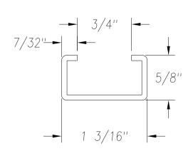
SEE PO FOR MATERIAL TYPE AND FINISH FOR LENGTH DIMENSION ("L"), SEE PURCHASE ORDER. LENGTH TOLERANCE:LESS THAN 60":  $\pm 1/16$ " LESS THAN 120":  $\pm 1/8$ ", 120" OR GREATER:  $\pm 1/4$ " MAXIMUM BURR NOT TO EXCEED 10% OF MAT'L THICKNESS WITH THE EXCEPTION OF CUT ENDS, WHICH MAY HAVE BURR EXCEEDING THIS AMOUNT. FINISHED PART MAY EXHIBIT TYPICAL ROLL FORMED END CUT DISTORTION. PROFILE DIMENSIONS TO BE MEASURED 2" OR GREATER FROM CUT ENDS.
