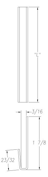
SEE PO FOR MATERIAL TYPE AND FINISH FOR LENGTH DIMENSION ("L"), SEE PURCHASE ORDER. LENGTH TOLERANCE:LESS THAN 60": ±1/16" LESS THAN 120": ±1/8", 120" OR GREATER: ± 1/4" MAXIMUM BURR NOT TO EXCEED 10% OF MAT'L THICKNESS WITH THE EXCEPTION OF CUT ENDS, WHICH MAY HAVE BURR EXCEEDING THIS AMOUNT. FINISHED PART MAY EXHIBIT TYPICAL ROLL FORMED END CUT DISTORTION. PROFILE DIMENSIONS TO BE MEASURED 2" OR GREATER FROM CUT ENDS.
