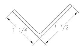
SEE PO FOR MATERIAL TYPE AND FINISH FOR LENGTH DIMENSION ("L"), SEE PURCHASE ORDER. LENGTH TOLERANCE:LESS THAN 60":  $\pm 1/16$ " LESS THAN 120":  $\pm 1/8$ ", 120" OR GREATER:  $\pm 1/4$ " MAXIMUM BURR NOT TO EXCEED 10% OF MAT'L THICKNESS WITH THE EXCEPTION OF CUT ENDS, WHICH MAY HAVE BURR EXCEEDING THIS AMOUNT. FINISHED PART MAY EXHIBIT TYPICAL ROLL FORMED END CUT DISTORTION. PROFILE DIMENSIONS TO BE MEASURED 2" OR GREATER FROM CUT ENDS.
