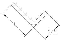
SEE PO FOR MATERIAL TYPE AND FINISH FOR LENGTH DIMENSION ("L"), SEE PURCHASE ORDER. LENGTH TOLERANCE:LESS THAN 60": ±1/16" LESS THAN 120": ±1/8", 120" OR GREATER: ± 1/4" MAXIMUM BURR NOT TO EXCEED 10% OF MAT'L THICKNESS WITH THE EXCEPTION OF CUT ENDS, WHICH MAY HAVE BURR EXCEEDING THIS AMOUNT. FINISHED PART MAY EXHIBIT TYPICAL ROLL FORMED END CUT DISTORTION. PROFILE DIMENSIONS TO BE MEASURED 2" OR GREATER FROM CUT ENDS.
