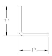
SEE PO FOR MATERIAL TYPE AND FINISH FOR LENGTH DIMENSION ("L"), SEE PURCHASE ORDER. LENGTH TOLERANCE:LESS THAN 60":  $\pm 1/16$ " LESS THAN 120":  $\pm 1/8$ ", 120" OR GREATER:  $\pm 1/4$ " MAXIMUM BURR NOT TO EXCEED 10% OF MAT'L THICKNESS WITH THE EXCEPTION OF CUT ENDS, WHICH MAY HAVE BURR EXCEEDING THIS AMOUNT. FINISHED PART MAY EXHIBIT TYPICAL ROLL FORMED END CUT DISTORTION. PROFILE DIMENSIONS TO BE MEASURED 2" OR GREATER FROM CUT ENDS.
