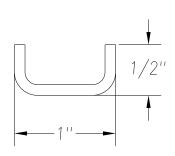
SEE PO FOR MATERIAL TYPE AND FINISH FOR LENGTH DIMENSION ("L"), SEE PURCHASE ORDER. LENGTH TOLERANCE:LESS THAN 60":  $\pm 1/16$ " LESS THAN 120":  $\pm 1/8$ ", 120" OR GREATER:  $\pm 1/4$ " MAXIMUM BURR NOT TO EXCEED 10% OF MAT'L THICKNESS WITH THE EXCEPTION OF CUT ENDS, WHICH MAY HAVE BURR EXCEEDING THIS AMOUNT. FINISHED PART MAY EXHIBIT TYPICAL ROLL FORMED END CUT DISTORTION. PROFILE DIMENSIONS TO BE MEASURED 2" OR GREATER FROM CUT ENDS.
