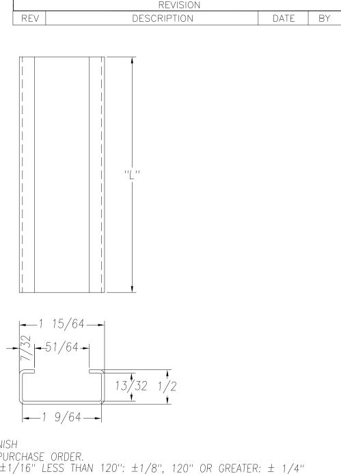
SEE PO FOR MATERIAL TYPE AND FINISH FOR LENGTH DIMENSION ("L"), SEE PURCHASE ORDER. LENGTH TOLERANCE:LESS THAN 60":  $\pm 1/16$ " LESS THAN 120":  $\pm 1/8$ ", 120" OR GREATER:  $\pm 1/4$ " MAXIMUM BURR NOT TO EXCEED 10% OF MAT'L THICKNESS WITH THE EXCEPTION OF CUT ENDS, WHICH MAY HAVE BURR EXCEEDING THIS AMOUNT. FINISHED PART MAY EXHIBIT TYPICAL ROLL FORMED END CUT DISTORTION. PROFILE DIMENSIONS TO BE MEASURED 2" OR GREATER FROM CUT ENDS.
