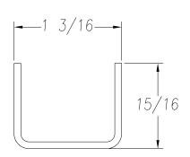
SEE PO FOR MATERIAL TYPE AND FINISH FOR LENGTH DIMENSION ("L"), SEE PURCHASE ORDER. LENGTH TOLERANCE:LESS THAN 60":  $\pm 1/16$ " LESS THAN 120":  $\pm 1/8$ ", 120" OR GREATER:  $\pm 1/4$ " MAXIMUM BURR NOT TO EXCEED 10% OF MAT'L THICKNESS WITH THE EXCEPTION OF CUT ENDS, WHICH MAY HAVE BURR EXCEEDING THIS AMOUNT. FINISHED PART MAY EXHIBIT TYPICAL ROLL FORMED END CUT DISTORTION. PROFILE DIMENSIONS TO BE MEASURED 2" OR GREATER FROM CUT ENDS.
