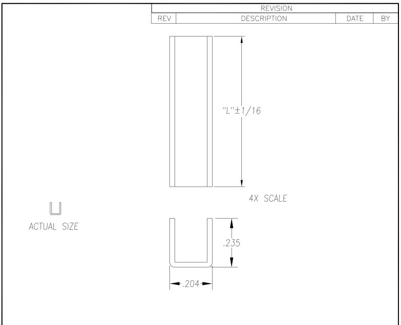
SEE PO FOR MATERIAL TYPE AND FINISH FOR LENGTH DIMENSION ("L"), SEE PURCHASE ORDER. LENGTH TOLERANCE:LESS THAN 60": ±1/16" LESS THAN 120": ±1/8", 120" OR GREATER: ± 1/4" MAXIMUM BURR NOT TO EXCEED 10% OF MAT'L THICKNESS WITH THE EXCEPTION OF CUT ENDS, WHICH MAY HAVE BURR EXCEEDING THIS AMOUNT. FINISHED PART MAY EXHIBIT TYPICAL ROLL FORMED END CUT DISTORTION. PROFILE DIMENSIONS TO BE MEASURED 2" OR GREATER FROM CUT ENDS.
