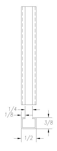
SEE PO FOR MATERIAL TYPE AND FINISH FOR LENGTH DIMENSION ("L"), SEE PURCHASE ORDER. LENGTH TOLERANCE:LESS THAN 60":  $\pm 1/16$ " LESS THAN 120":  $\pm 1/8$ ", 120" OR GREATER:  $\pm 1/4$ " MAXIMUM BURR NOT TO EXCEED 10% OF MAT'L THICKNESS WITH THE EXCEPTION OF CUT ENDS, WHICH MAY HAVE BURR EXCEEDING THIS AMOUNT. FINISHED PART MAY EXHIBIT TYPICAL ROLL FORMED END CUT DISTORTION. PROFILE DIMENSIONS TO BE MEASURED 2" OR GREATER FROM CUT ENDS.
