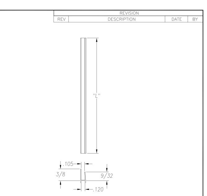
SEE PO FOR MATERIAL TYPE AND FINISH FOR LENGTH DIMENSION ("L"), SEE PURCHASE ORDER. LENGTH TOLERANCE:LESS THAN 60":  $\pm 1/16$ " LESS THAN 120":  $\pm 1/8$ ", 120" OR GREATER:  $\pm 1/4$ " MAXIMUM BURR NOT TO EXCEED 10% OF MAT'L THICKNESS WITH THE EXCEPTION OF CUT ENDS, WHICH MAY HAVE BURR EXCEEDING THIS AMOUNT. FINISHED PART MAY EXHIBIT TYPICAL ROLL FORMED END CUT DISTORTION. PROFILE DIMENSIONS TO BE MEASURED 2" OR GREATER FROM CUT ENDS.
