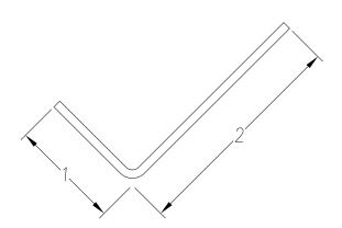
SEE PO FOR MATERIAL TYPE AND FINISH FOR LENGTH DIMENSION ("L"), SEE PURCHASE ORDER. LENGTH TOLERANCE:LESS THAN 60":  $\pm 1/16$ " LESS THAN 120":  $\pm 1/8$ ", 120" OR GREATER:  $\pm 1/4$ " MAXIMUM BURR NOT TO EXCEED 10% OF MAT'L THICKNESS WITH THE EXCEPTION OF CUT ENDS, WHICH MAY HAVE BURR EXCEEDING THIS AMOUNT. FINISHED PART MAY EXHIBIT TYPICAL ROLL FORMED END CUT DISTORTION. PROFILE DIMENSIONS TO BE MEASURED 2" OR GREATER FROM CUT ENDS.
