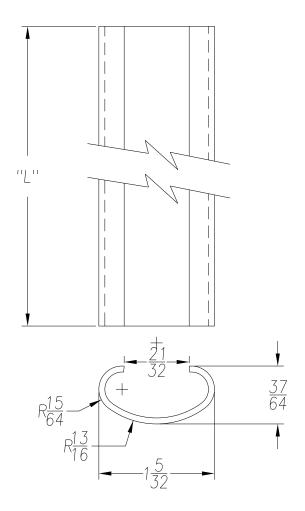
SEE PO FOR MATERIAL TYPE AND FINISH FOR LENGTH DIMENSION ("L"), SEE PURCHASE ORDER. LENGTH TOLERANCE:LESS THAN 60": ±1/16" LESS THAN 120": ±1/8", 120" OR GREATER: ± 1/4" MAXIMUM BURR NOT TO EXCEED 10% OF MAT'L THICKNESS WITH THE EXCEPTION OF CUT ENDS, WHICH MAY HAVE BURR EXCEEDING THIS AMOUNT. FINISHED PART MAY EXHIBIT TYPICAL ROLL FORMED END CUT DISTORTION. PROFILE DIMENSIONS TO BE MEASURED 2" OR GREATER FROM CUT ENDS.
