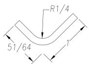
SEE PO FOR MATERIAL TYPE AND FINISH FOR LENGTH DIMENSION ("L"), SEE PURCHASE ORDER. LENGTH TOLERANCE:LESS THAN 60":  $\pm 1/16$ " LESS THAN 120":  $\pm 1/8$ ", 120" OR GREATER:  $\pm 1/4$ " MAXIMUM BURR NOT TO EXCEED 10% OF MAT'L THICKNESS WITH THE EXCEPTION OF CUT ENDS, WHICH MAY HAVE BURR EXCEEDING THIS AMOUNT. FINISHED PART MAY EXHIBIT TYPICAL ROLL FORMED END CUT DISTORTION. PROFILE DIMENSIONS TO BE MEASURED 2" OR GREATER FROM CUT ENDS.
