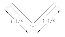
SEE PO FOR MATERIAL TYPE AND FINISH FOR LENGTH DIMENSION ("L"), SEE PURCHASE ORDER. LENGTH TOLERANCE:LESS THAN 60": ±1/16" LESS THAN 120": ±1/8", 120" OR GREATER: ± 1/4" MAXIMUM BURR NOT TO EXCEED 10% OF MAT'L THICKNESS WITH THE EXCEPTION OF CUT ENDS, WHICH MAY HAVE BURR EXCEEDING THIS AMOUNT. FINISHED PART MAY EXHIBIT TYPICAL ROLL FORMED END CUT DISTORTION. PROFILE DIMENSIONS TO BE MEASURED 2" OR GREATER FROM CUT ENDS.
