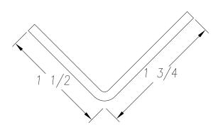
SEE PO FOR MATERIAL TYPE AND FINISH FOR LENGTH DIMENSION ("L"), SEE PURCHASE ORDER. LENGTH TOLERANCE:LESS THAN 60":  $\pm 1/16$ " LESS THAN 120":  $\pm 1/8$ ", 120" OR GREATER:  $\pm 1/4$ " MAXIMUM BURR NOT TO EXCEED 10% OF MAT'L THICKNESS WITH THE EXCEPTION OF CUT ENDS, WHICH MAY HAVE BURR EXCEEDING THIS AMOUNT. FINISHED PART MAY EXHIBIT TYPICAL ROLL FORMED END CUT DISTORTION. PROFILE DIMENSIONS TO BE MEASURED 2" OR GREATER FROM CUT ENDS.
