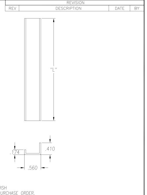
SEE PO FOR MATERIAL TYPE AND FINISH FOR LENGTH DIMENSION ("L"), SEE PURCHASE ORDER. LENGTH TOLERANCE:LESS THAN 60":  $\pm 1/16$ " LESS THAN 120":  $\pm 1/8$ ", 120" OR GREATER:  $\pm 1/4$ " MAXIMUM BURR NOT TO EXCEED 10% OF MAT'L THICKNESS WITH THE EXCEPTION OF CUT ENDS, WHICH MAY HAVE BURR EXCEEDING THIS AMOUNT. FINISHED PART MAY EXHIBIT TYPICAL ROLL FORMED END FLARE UP TO THREE INCHES FROM ENDS. PROFILE DIMENSIONS TO BE MEASURED 3" OR GREATER FROM CUT ENDS.
