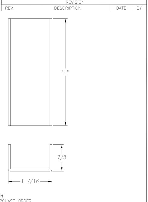
SEE PO FOR MATERIAL TYPE AND FINISH FOR LENGTH DIMENSION ("L"), SEE PURCHASE ORDER. LENGTH TOLERANCE:LESS THAN 60": ±1/16" LESS THAN 120": ±1/8", 120" OR GREATER: ± 1/4" MAXIMUM BURR NOT TO EXCEED 10% OF MAT'L THICKNESS WITH THE EXCEPTION OF CUT ENDS, WHICH MAY HAVE BURR EXCEEDING THIS AMOUNT. FINISHED PART MAY EXHIBIT TYPICAL ROLL FORMED END FLARE UP TO THREE INCHES FROM ENDS. PROFILE DIMENSIONS TO BE MEASURED 3" OR GREATER FROM CUT ENDS.
