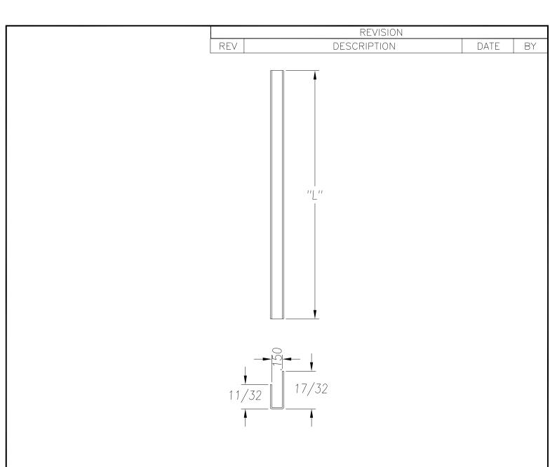
SEE PO FOR MATERIAL TYPE AND FINISH FOR LENGTH DIMENSION ("L"), SEE PURCHASE ORDER. LENGTH TOLERANCE:LESS THAN 60":  $\pm 1/16$ " LESS THAN 120":  $\pm 1/8$ ", 120" OR GREATER:  $\pm 1/4$ " MAXIMUM BURR NOT TO EXCEED 10% OF MAT'L THICKNESS WITH THE EXCEPTION OF CUT ENDS, WHICH MAY HAVE BURR EXCEEDING THIS AMOUNT. FINISHED PART MAY EXHIBIT TYPICAL ROLL FORMED END FLARE UP TO THREE INCHES FROM ENDS. PROFILE DIMENSIONS TO BE MEASURED 3" OR GREATER FROM CUT ENDS.
