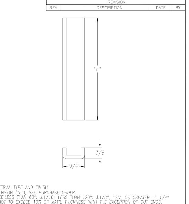
SEE PO FOR MATERIAL TYPE AND FINISH FOR LENGTH DIMENSION ("L"), SEE PURCHASE ORDER. LENGTH TOLERANCE:LESS THAN 60": ±1/16" LESS THAN 120": ±1/8", 120" OR GREATER: ± 1/4" MAXIMUM BURR NOT TO EXCEED 10% OF MAT'L THICKNESS WITH THE EXCEPTION OF CUT ENDS, WHICH MAY HAVE BURR EXCEEDING THIS AMOUNT. FINISHED PART MAY EXHIBIT TYPICAL ROLL FORMED END FLARE UP TO THREE INCHES FROM ENDS. PROFILE DIMENSIONS TO BE MEASURED 3" OR GREATER FROM CUT ENDS.
