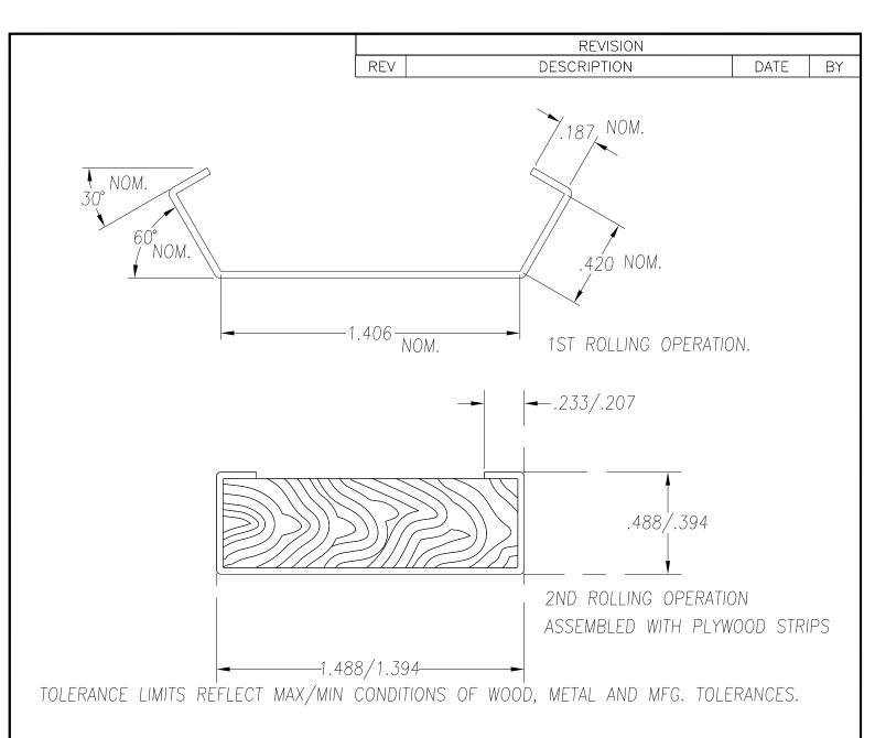
SEE PO FOR MATERIAL TYPE AND FINISH FOR LENGTH DIMENSION ("L"), SEE PURCHASE ORDER. LENGTH TOLERANCE:LESS THAN 60":  $\pm 1/16$ " LESS THAN 120":  $\pm 1/8$ ", 120" OR GREATER:  $\pm 1/4$ " MAXIMUM BURR NOT TO EXCEED 10% OF MAT'L THICKNESS WITH THE EXCEPTION OF CUT ENDS, WHICH MAY HAVE BURR EXCEEDING THIS AMOUNT. FINISHED PART MAY EXHIBIT TYPICAL ROLL FORMED END CUT DISTORTION. PROFILE DIMENSIONS TO BE MEASURED 2" OR GREATER FROM CUT ENDS.
