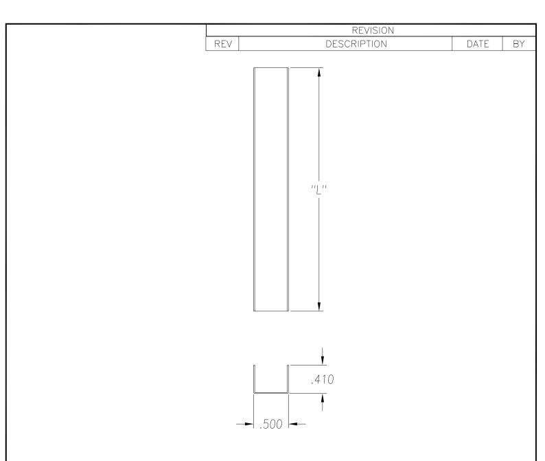
SEE PO FOR MATERIAL TYPE AND FINISH FOR LENGTH DIMENSION ("L"), SEE PURCHASE ORDER. LENGTH TOLERANCE:LESS THAN 60":  $\pm 1/16$ " LESS THAN 120":  $\pm 1/8$ ", 120" OR GREATER:  $\pm 1/4$ " MAXIMUM BURR NOT TO EXCEED 10% OF MAT'L THICKNESS WITH THE EXCEPTION OF CUT ENDS, WHICH MAY HAVE BURR EXCEEDING THIS AMOUNT. FINISHED PART MAY EXHIBIT TYPICAL ROLL FORMED END FLARE UP TO THREE INCHES FROM ENDS. PROFILE DIMENSIONS TO BE MEASURED 3" OR GREATER FROM CUT ENDS.
