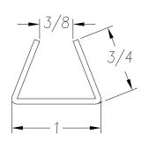
SEE PO FOR MATERIAL TYPE AND FINISH FOR LENGTH DIMENSION ("L"), SEE PURCHASE ORDER. LENGTH TOLERANCE:LESS THAN 60":  $\pm 1/16$ " LESS THAN 120":  $\pm 1/8$ ", 120" OR GREATER:  $\pm 1/4$ " MAXIMUM BURR NOT TO EXCEED 10% OF MAT'L THICKNESS WITH THE EXCEPTION OF CUT ENDS, WHICH MAY HAVE BURR EXCEEDING THIS AMOUNT. FINISHED PART MAY EXHIBIT TYPICAL ROLL FORMED END FLARE UP TO THREE INCHES FROM ENDS. PROFILE DIMENSIONS TO BE MEASURED 3" OR GREATER FROM CUT ENDS.
