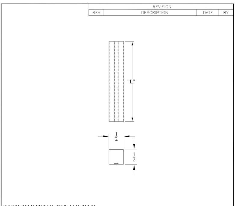
SEE PO FOR MATERIAL TYPE AND FINISH FOR LENGTH DIMENSION ("L"), SEE PURCHASE ORDER. LENGTH TOLERANCE:LESS THAN 60": ±1/16" LESS THAN 120": ±1/8", 120" OR GREATER: ± 1/4" MAXIMUM BURR NOT TO EXCEED 10% OF MAT'L THICKNESS WITH THE EXCEPTION OF CUT ENDS, WHICH MAY HAVE BURR EXCEEDING THIS AMOUNT. FINISHED PART MAY EXHIBIT TYPICAL ROLL FORMED END FLARE UP TO THREE INCHES FROM ENDS. PROFILE DIMENSIONS TO BE MEASURED 3" OR GREATER FROM CUT ENDS.
