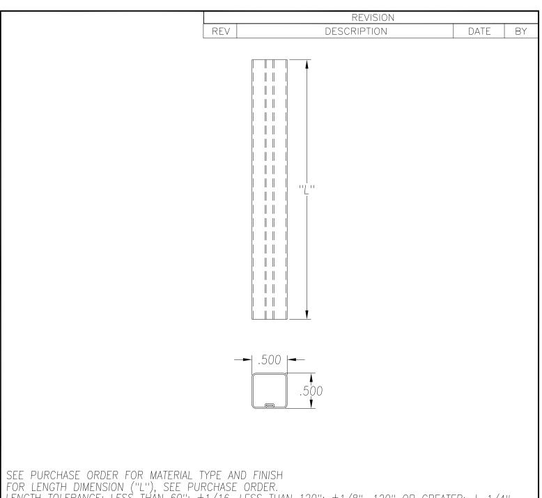
SEE PURCHASE ORDER FOR MATERIAL TYPE AND FINISH FOR LENGTH DIMENSION ("L"), SEE PURCHASE ORDER. LENGTH TOLERANCE: LESS THAN 60": ±1/16, LESS THAN 120": ±1/8", 120" OR GREATER: ± 1/4" MAXIMUM BURR NOT TO EXCEED 10% OF MAT'L THICKNESS WITH THE EXCEPTION OF CUT ENDS, WHICH MAY HAVE BURR EXCEEDING THIS AMOUNT. PROFILE DIMENSIONS TO BE MEASURED 3" OR GREATER FROM CUT ENDS.
