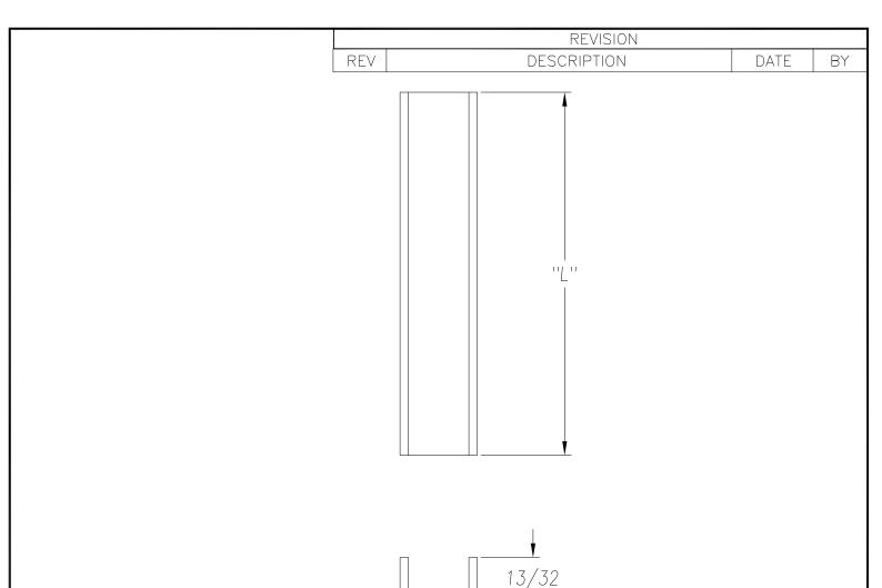
SEE PO FOR MATERIAL TYPE AND FINISH FOR LENGTH DIMENSION ("L"), SEE PURCHASE ORDER. LENGTH TOLERANCE:LESS THAN 60": ±1/16" LESS THAN 120": ±1/8", 120" OR GREATER: ± 1/4" MAXIMUM BURR NOT TO EXCEED 10% OF MAT'L THICKNESS WITH THE EXCEPTION OF CUT ENDS, WHICH MAY HAVE BURR EXCEEDING THIS AMOUNT. FINISHED PART MAY EXHIBIT TYPICAL ROLL FORMED END FLARE UP TO THREE INCHES FROM ENDS. PROFILE DIMENSIONS TO BE MEASURED 3" OR GREATER FROM CUT ENDS.
