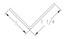
SEE PO FOR MATERIAL TYPE AND FINISH FOR LENGTH DIMENSION ("L"), SEE PURCHASE ORDER. LENGTH TOLERANCE:LESS THAN 60": ±1/16" LESS THAN 120": ±1/8", 120" OR GREATER: ± 1/4" MAXIMUM BURR NOT TO EXCEED 10% OF MAT'L THICKNESS WITH THE EXCEPTION OF CUT ENDS, WHICH MAY HAVE BURR EXCEEDING THIS AMOUNT. FINISHED PART MAY EXHIBIT TYPICAL ROLL FORMED END FLARE UP TO THREE INCHES FROM ENDS. PROFILE DIMENSIONS TO BE MEASURED 3" OR GREATER FROM CUT ENDS.
