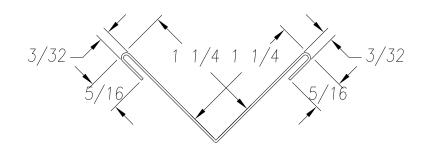
SEE PO FOR MATERIAL TYPE AND FINISH FOR LENGTH DIMENSION ("L"), SEE PURCHASE ORDER. LENGTH TOLERANCE:LESS THAN 60":  $\pm 1/16$ " LESS THAN 120":  $\pm 1/8$ ", 120" OR GREATER:  $\pm 1/4$ " MAXIMUM BURR NOT TO EXCEED 10% OF MAT'L THICKNESS WITH THE EXCEPTION OF CUT ENDS, WHICH MAY HAVE BURR EXCEEDING THIS AMOUNT.
