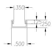
SEE PO FOR MATERIAL TYPE AND FINISH FOR LENGTH DIMENSION ("L"), SEE PURCHASE ORDER. LENGTH TOLERANCE:LESS THAN 60":  $\pm 1/16$ " LESS THAN 120":  $\pm 1/8$ ", 120" OR GREATER:  $\pm 1/4$ " MAXIMUM BURR NOT TO EXCEED 10% OF MAT'L THICKNESS WITH THE EXCEPTION OF CUT ENDS, WHICH MAY HAVE BURR EXCEEDING THIS AMOUNT. FINISHED PART MAY EXHIBIT TYPICAL ROLL FORMED END FLARE UP TO THREE INCHES FROM ENDS. PROFILE DIMENSIONS TO BE MEASURED 3" OR GREATER FROM CUT ENDS.
