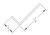
SEE PURCHASE ORDER FOR MATERIAL TYPE AND FINISH FOR LENGTH DIMENSION ("L"), SEE PURCHASE ORDER. LENGTH TOLERANCE: LESS THAN 60":  $\pm 1/16$ , LESS THAN 120":  $\pm 1/8$ ", 120" OR GREATER:  $\pm 1/4$ " MAXIMUM BURR NOT TO EXCEED 10% OF MAT'L THICKNESS WITH THE EXCEPTION OF CUT ENDS, WHICH MAY HAVE BURR EXCEEDING THIS AMOUNT. PROFILE MAY EXHIBIT TYPICAL ROLL FORMED END FLARE UP TO 3" FROM ENDS. PART TO BE MEASURED 3" OR GREATER FROM CUT ENDS.
