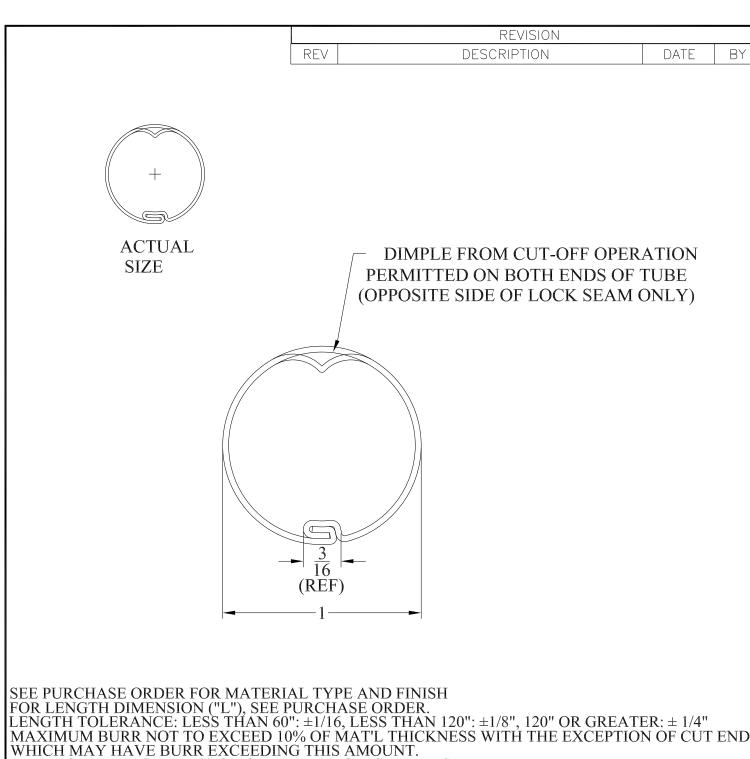
SEE PURCHASE ORDER FOR MATERIAL TYPE AND FINISH FOR LENGTH DIMENSION ("L"), SEE PURCHASE ORDER. LENGTH TOLERANCE: LESS THAN 60": ±1/16, LESS THAN 120": ±1/8", 120" OR GREATER: ± 1/4" MAXIMUM BURR NOT TO EXCEED 10% OF MAT'L THICKNESS WITH THE EXCEPTION OF CUT ENDS, WHICH MAY HAVE BURR EXCEEDING THIS AMOUNT. PART TO BE MEASURED 3" OR GREATER FROM CUT ENDS.
