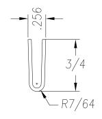
SEE PO FOR MATERIAL TYPE AND FINISH FOR LENGTH DIMENSION ("L"), SEE PURCHASE ORDER. LENGTH TOLERANCE:LESS THAN 60":  $\pm 1/16$ " LESS THAN 120":  $\pm 1/8$ ", 120" OR GREATER:  $\pm 1/4$ " MAXIMUM BURR NOT TO EXCEED 10% OF MAT'L THICKNESS WITH THE EXCEPTION OF CUT ENDS, WHICH MAY HAVE BURR EXCEEDING THIS AMOUNT. FINISHED PART MAY EXHIBIT TYPICAL ROLL FORMED END FLARE UP TO THREE INCHES FROM ENDS. PROFILE DIMENSIONS TO BE MEASURED 3" OR GREATER FROM CUT ENDS.
