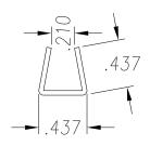
SEE PO FOR MATERIAL TYPE AND FINISH FOR LENGTH DIMENSION ("L"), SEE PURCHASE ORDER. LENGTH TOLERANCE:LESS THAN 60": ±1/16" LESS THAN 120": ±1/8", 120" OR GREATER: ± 1/4" MAXIMUM BURR NOT TO EXCEED 10% OF MAT'L THICKNESS WITH THE EXCEPTION OF CUT ENDS, WHICH MAY HAVE BURR EXCEEDING THIS AMOUNT. FINISHED PART MAY EXHIBIT TYPICAL ROLL FORMED END FLARE UP TO THREE INCHES FROM ENDS. PROFILE DIMENSIONS TO BE MEASURED 3" OR GREATER FROM CUT ENDS.
